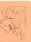
The first tray is a catchment or corner tray. Bed on mortar in the lowest appropriate course. Slide the tray to the left or right, until the corner is 75mm\* above the finished
